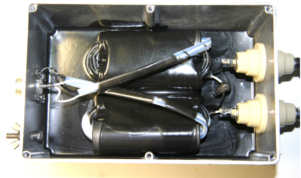
Fig 38 –Choke (Guanella) Transformer
