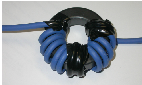
Fig 4 – A toroidal ferrite choke
